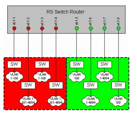
The above diagram depicts a complex scenario where a higher touch service is required to ensure broadcast domains within the logical administrative domains are maintained. In the 'Red' domain all user switches need to receive the default VLAN (1) untagged, but only two switches need VLANs 2-100, and the other two require only 101-4094. In the 'Green' domain all switches need the VLAN 100 untagged, but only two switches within the domain require the rest of the VLANs.
