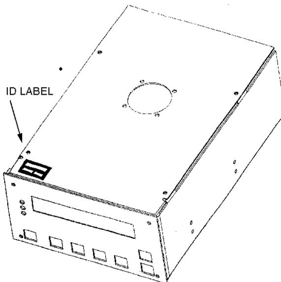
**Figure 1-2. Controller Identification Label**
