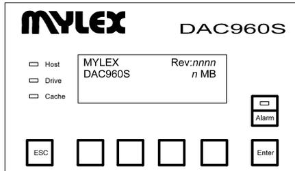
Figure 3-1. DAC960SI Front Panel Keypad and LCD
