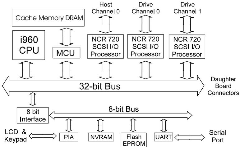
**Figure 2-2. Controller Block Diagram**
