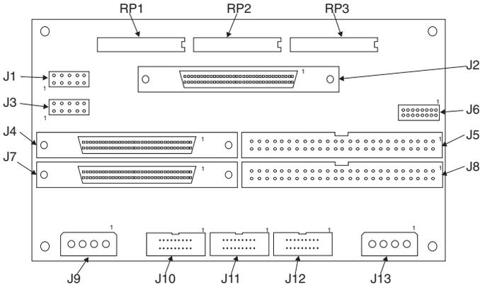
**Figure 1-5. DAC960SI-2D-n Differential SCSI Distribution Board**
