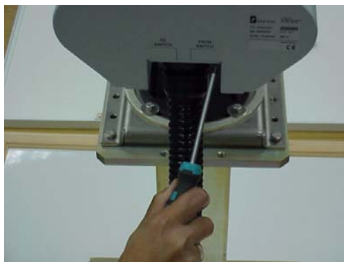
Disconnecting the flange and cable duct
