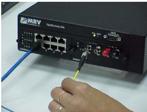
Connecting one end of the Transmit fiber to the TX port.
