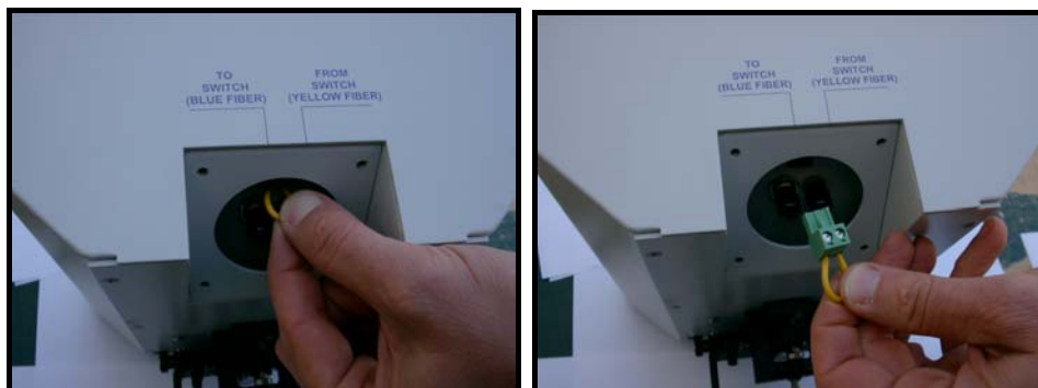
Figure 25: Extracting the Terminal Block by the Yellow Wire Loop
