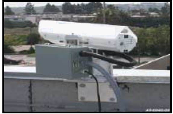
Figure 2.11: Angle Bracket Mounting (using JMP-L and M001)
