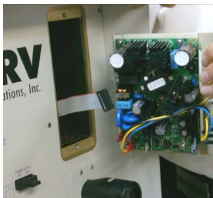
Figure I.3: Disconnected Flat Cable
