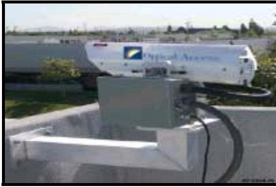
Figure 2.10: Extended Wall Mounting (using JMP and MO62C)
