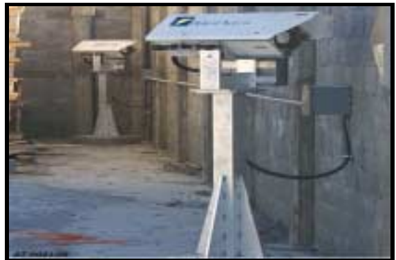
Figure 2.7: Floor Pedestal Mounting (using JMP and MO15C)
