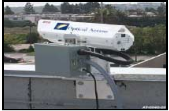
Figure 2.11: Angle Bracket Mounting (using JMP and M001)
