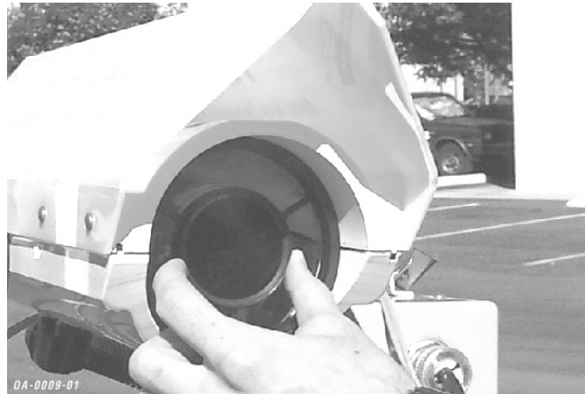
Figure C-5. Threading the neutral density filter into the mount.
