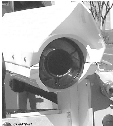
Figure C-6. Attenuator mount and neutral density filter correctly installed.
