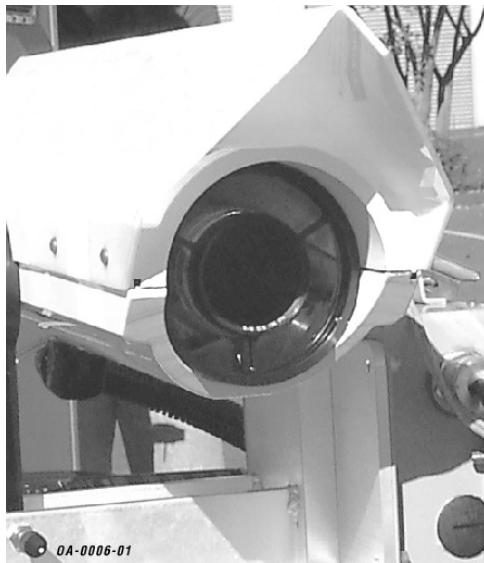
Figure 11. Placement of neutral density filters over the transmit aperture prevents saturation of the detector at close, demonstration-type ranges.
