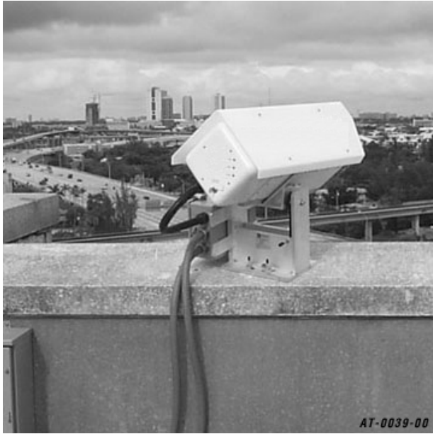
Figure B-1. Mountable Gimbal - Direct to a flat wall surface. Attach with 4-3/8" concrete anchors.
