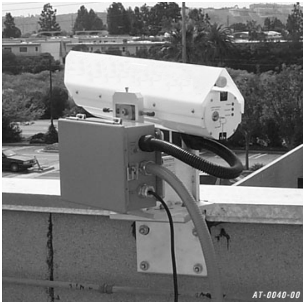
Figure B-2. M001 Angle Bracket - Use when the wall is too thin to mount to the top. Can be used on inner or outer wall surface (reversible).
