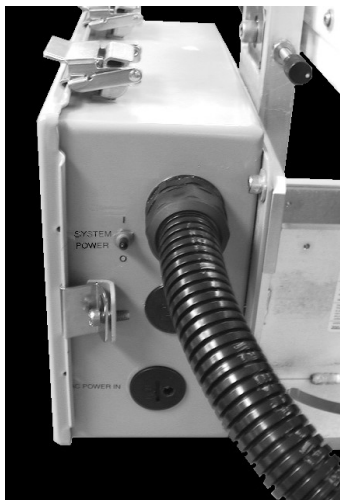
Figure 5. Location of the power switch at the back of the electronics box.
