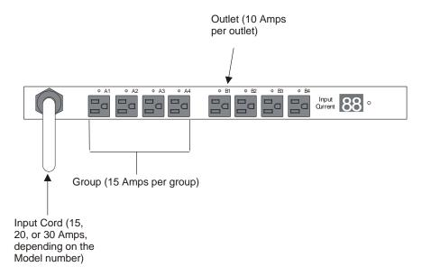
Figure 1 – 120V 5150 Power Control Series Amperage Issues
