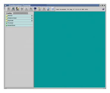
2. To log in as a superuser, click the **Admin** button on the tool bar and log in with the default Superuser password system. You can now configure the unit via the GUI.
