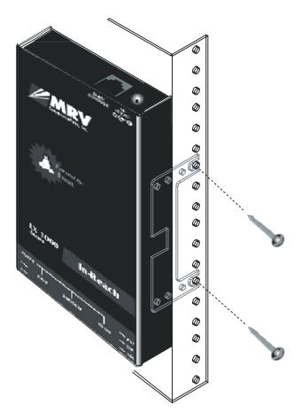
Figure 7 - Side-Mounting an LX-1000 Series in a Rack
