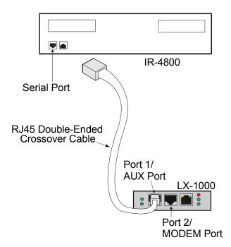
Figure 17 - Connecting the IR-4800
