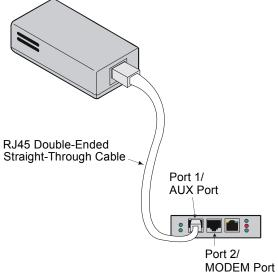
Figure 15 - Connecting the Temperature/Humidity Sensor
