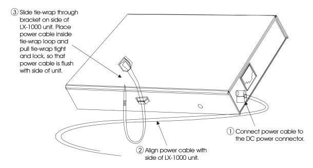
Figure 12 - Attaching the Tie-Wrap
