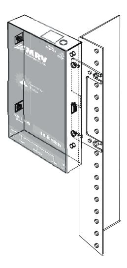
Figure 8 - Front-Mounting an LX-1000 Series in a Rack
