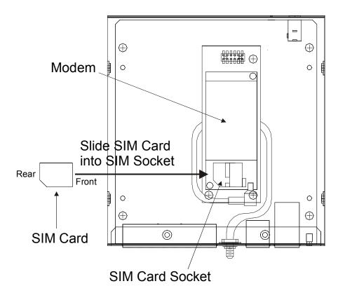
5. Locate the SIM Card socket on the GPRS Modem inside the LX-1000.
