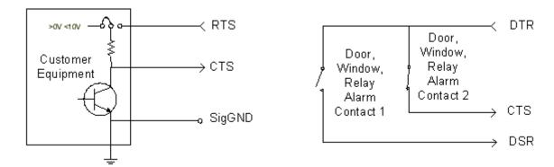
Figure 18 - Typical Alarm Inputs Connections
