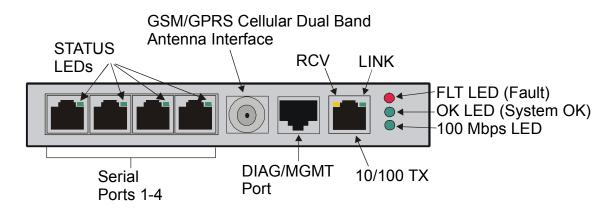
Figure 4 - LX-1000 Front Panel with Cellular Dual Band Antenna Interface
