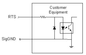
Figure 19 - Typical Interface Design for Control Output Signals
