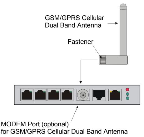
Figure 13 - Connecting the Cellular Dual Band Antenna
