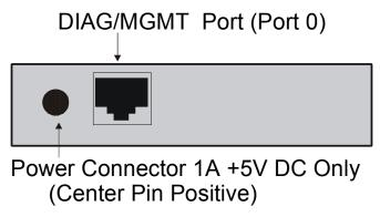
Figure 5 - LX-1000 Series 1- and 2-Port Rear Panel
