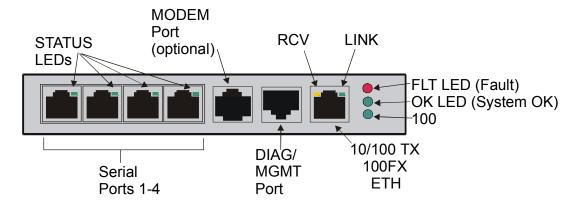
Figure 2 - LX-1000 Series 4-Port Front Panel
