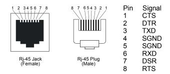
Figure 20 - Serial Device Connector (RJ-45) Signal Assignments
