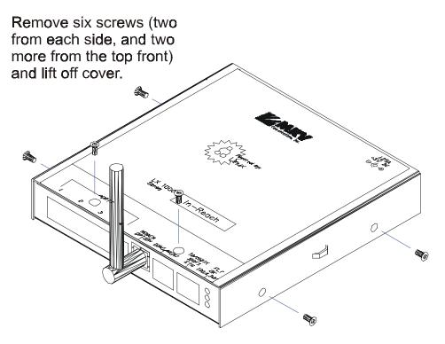
Figure 26 - Removing the Cover
