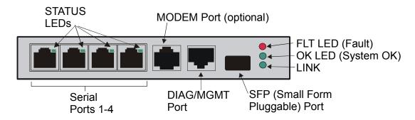
Figure 3 - LX-1000 Front Panel with SFP (Small Form-Factor Pluggable) Slot
