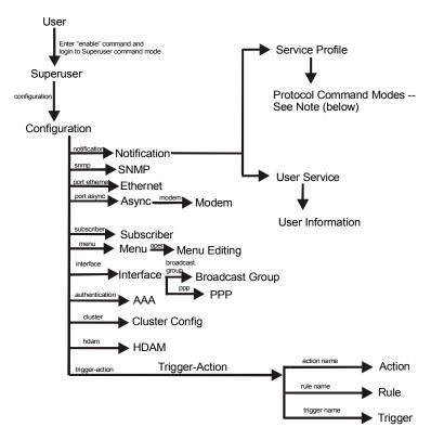
Note: The Protocol Command Modes include Async, Localsyslog, Remotesyslog, SMTP, SNPP, TAP, and WEB.
