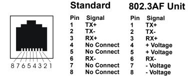
Figure 21 - 10/100 Connector Assignments
