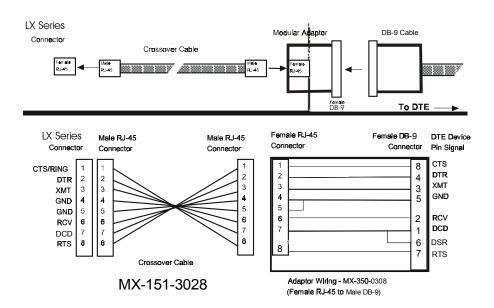
Figure 23 - Adapter Wiring, RJ-45 to DB-9, LX-1000 Series to DTE
