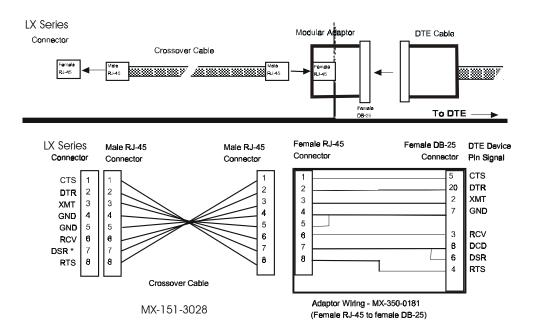
Figure 22 - Adapter Wiring, LX-1000 Series to DTE
