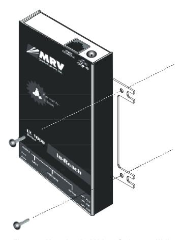
Figure 9 - Mounting the LX-1000 Series on a Wall
