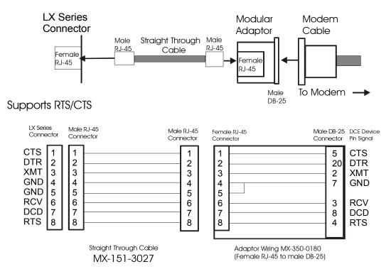
Figure 24 - Adapter Wiring, LX-1000 Series to DCE
