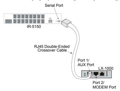
Figure 16 - Connecting the IR-5150
