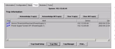
The Traps folder displays a message (SNMP Trap) indicating that Power Supply A has been turned off. A message can also be sent if the power supply goes above or below the acceptable voltage range.
