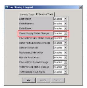
The Power Supply Status Change Traps is an Enterprise Trap and may be enabled or disabled.
