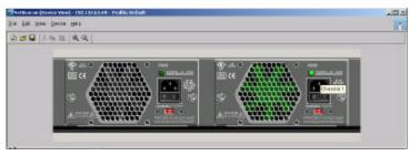
Power supply A has been disconnected. The fan has stopped running no longer shows as green.
