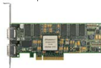
MHEA28-1TC – Dual 10Gb/s InfiniBand 128MB local SDRAM w/ PCI Express x8
