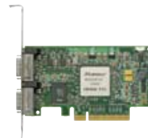
MHGA28-XTC –Dual 20Gb/s InfiniBand MemFree w/ PCI Express x8
