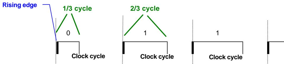
To convert from fiber to copper, an output clock is produced which identifies the beginning of each cycle and is cleared in the middle of each cycle. The PWM data value is sampled and NRZ output data is generated. During normal operation, the transmit (TX) and receive (RX) paths are clocked independently. If a receive line fails, the TDM interface generates a local clock to keep the transmit line alive.
