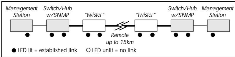
If the fiber connection breaks, or the remote device fails, the “twister” media converter carries that link loss all the way to the switch/hub which generates a trap to the management station. The administrator can then look at the media converter to determine the source of the loss.
