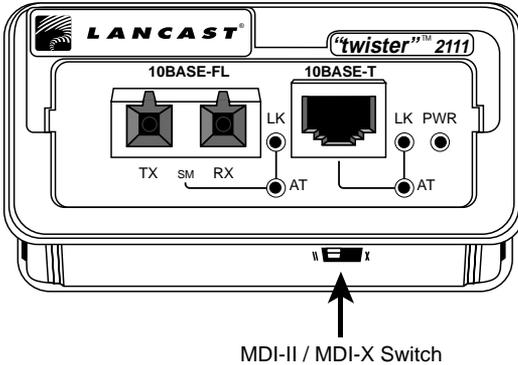
When setting the MDI-II to MDI-X switch, observe the positioning of the following symbols:
