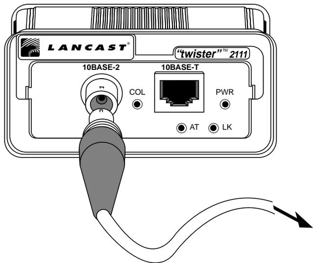
**IMPORTANT:** The coaxial cable of a LAN must be properly terminated at each end regardless of the device used at the end of each cable. A BNC terminator must be attached to each end of each trunk segment. One of the two terminators on each segment must be grounded. Refer to the illustration below:
