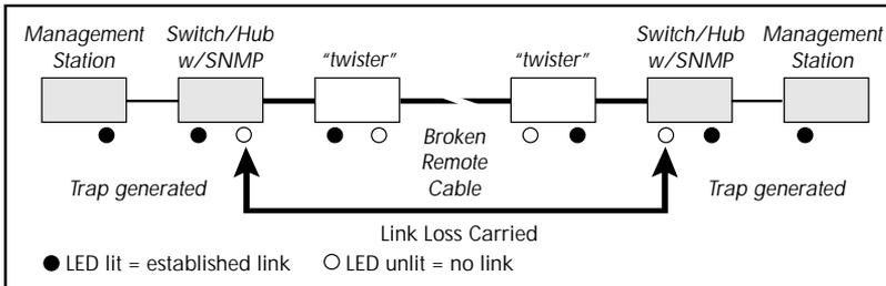
**IMPORTANT:** When connecting a “twister” media converter with LLCF enabled to an auto-negotiating device, force both sides of the configuration to either 10 or 100Mbps full or half duplex. This allows the media converter to immediately see link pulses and start passing data.
