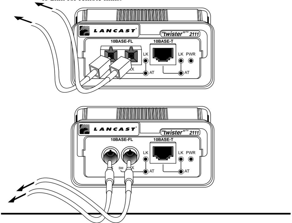
When making fiber optic connections, be sure that the transmit (TX) port of the “twister” connects to the receive (RX) port of the connected device; and be sure that the transmit (TX) port of the connected device connects to the receive (RX) port of the “twister” unit.
