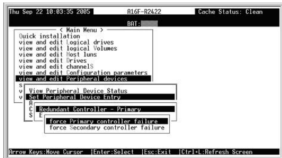
Figure 12 – 19 Redundant Controller testing
