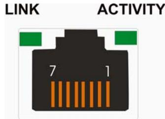
Figure C-7: Ethernet Port Pinouts
