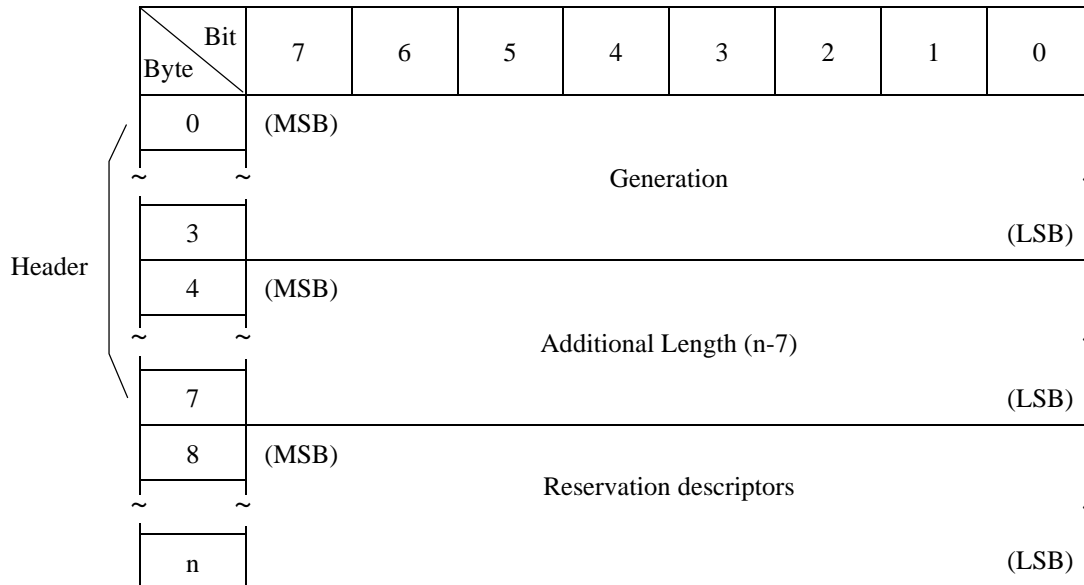
Figure 3.16 PERSISTENT RESERVE IN command: parameter data (READ RESERVATIONS)
