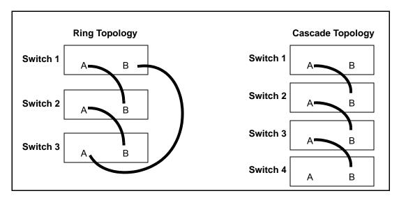
Figure 5 S50 Stacking Topologies
