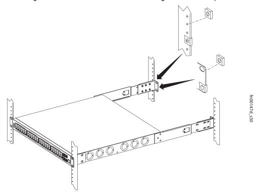
5. Align the rack filler panel to the rear bracket and rack posts. Secure by inserting two screws into the hole in the filler panel through to the holes in the rack post.
