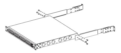
2. Insert the S50 into the rack, and secure the chassis to the front post with two screws. Then secure the chassis to the rear posts with two screws.
