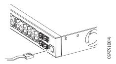
Figure 13 Front View of S50 Showing Console Port
