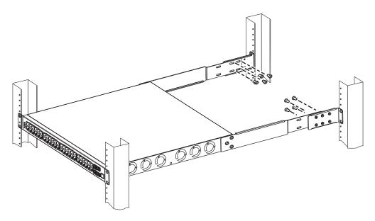
Figure 4 Four-post Rack-mounting with Adjustable Rear-mounting Brackets
