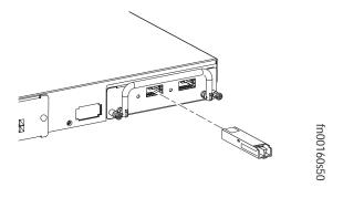
Figure 15 Rear View of S50 with XFP
