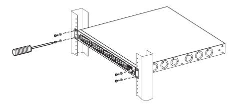
Figure 3 S50 Two-post (Front-mounted) Rack-mounting
