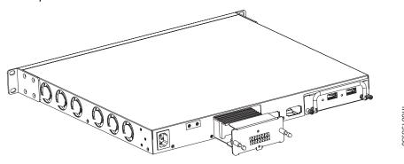
Figure 10 S50 Rear View Showing DC Power Module
