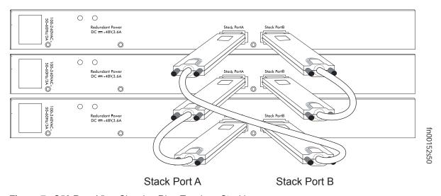
Figure 7 S50 Rear View Showing Ring Topology Stacking
