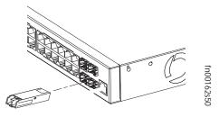
Figure 14 Front View of S50 with SFP
