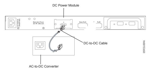
Figure 11 AC-DC Converter Connected to DC Power Module
