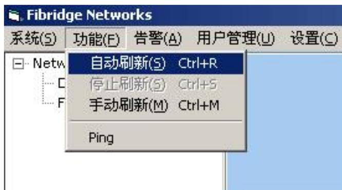
Refresh process displays the status information of each module and currently controlled module in real time. Each slot with module or not, the type number of each module and chassis display in the tree-like catalogue left of the windows. The status of the power supply displays below the display of the chassis.
