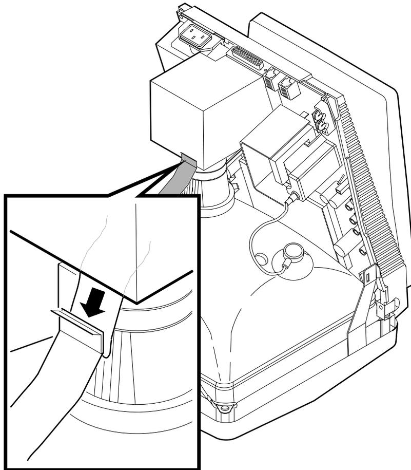
6. If you have a worldwide model, loosen the two screws securing the hood and remove the hood.
