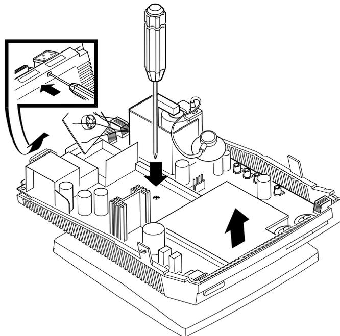
6. Pull the board away from the plastic tab on the connector side of the terminal board. You can release the tab by inserting a screwdriver through the hole below the tab.
