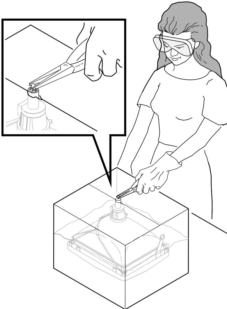
2. Seal up the container so that only the very tip of the CRT neck is exposed.
