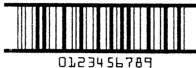
Figure F-2. Interleaved 2 of 5 Bar Code
