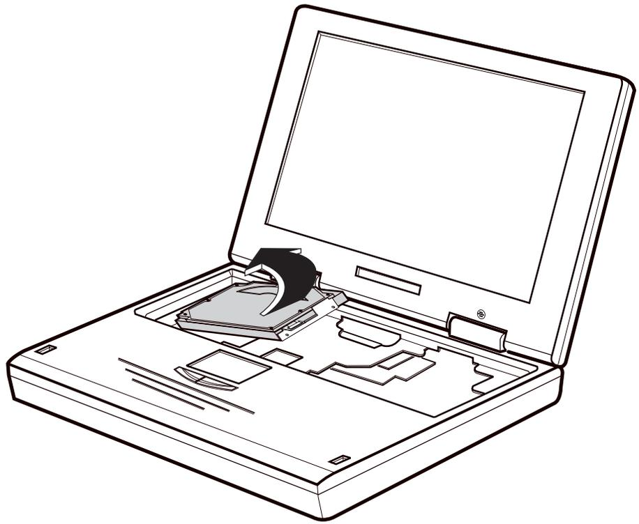
**Figure 4-6 Removing the Hard Drive**
