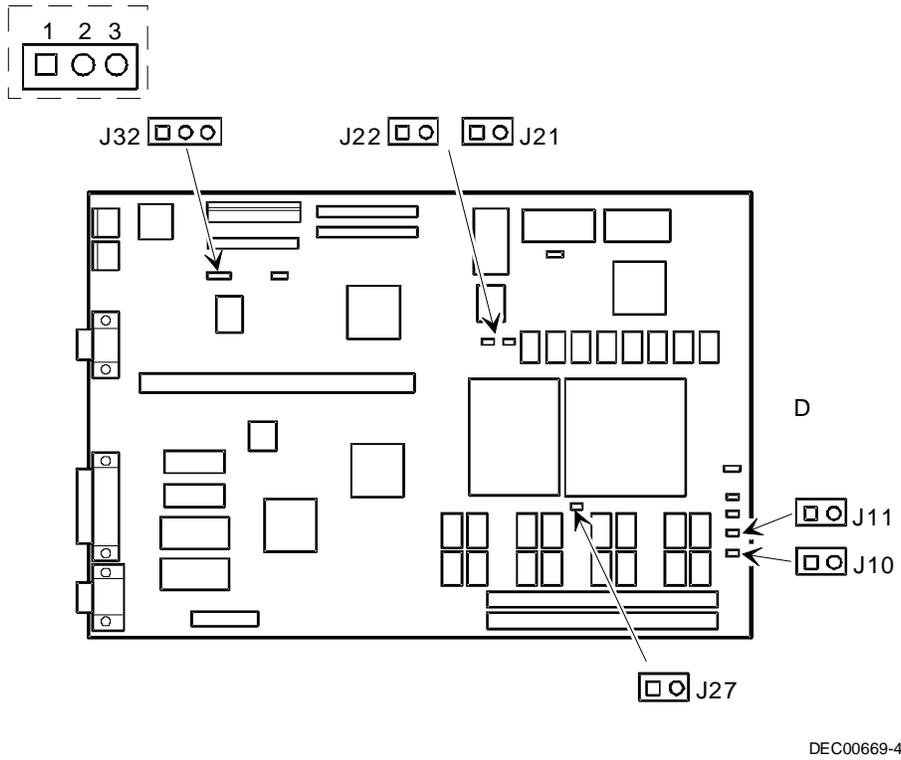
Figure 3 - 4 Main Logic Board Jumper Locations
