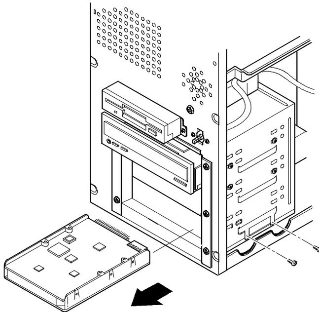
Figure 3 - 8 Removing the IDE Hard Disk Drive
