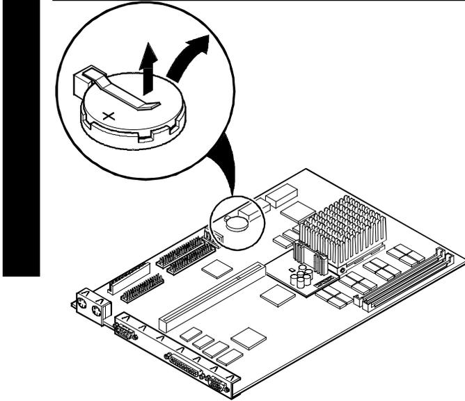
Figure 3 - 16 Replacing the Computer Battery
