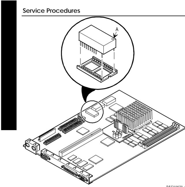
**Figure 3 - 15 Replacing the Real-Time Clock (RTC)**
