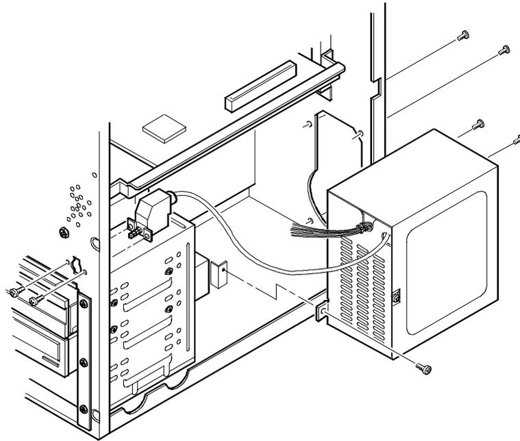
Figure 3 - 11 Removing the Power Supply
