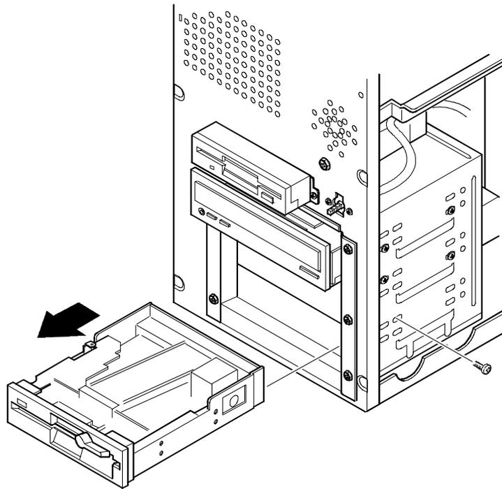
Figure 3 - 7 Removing a 5¼-Inch Device
