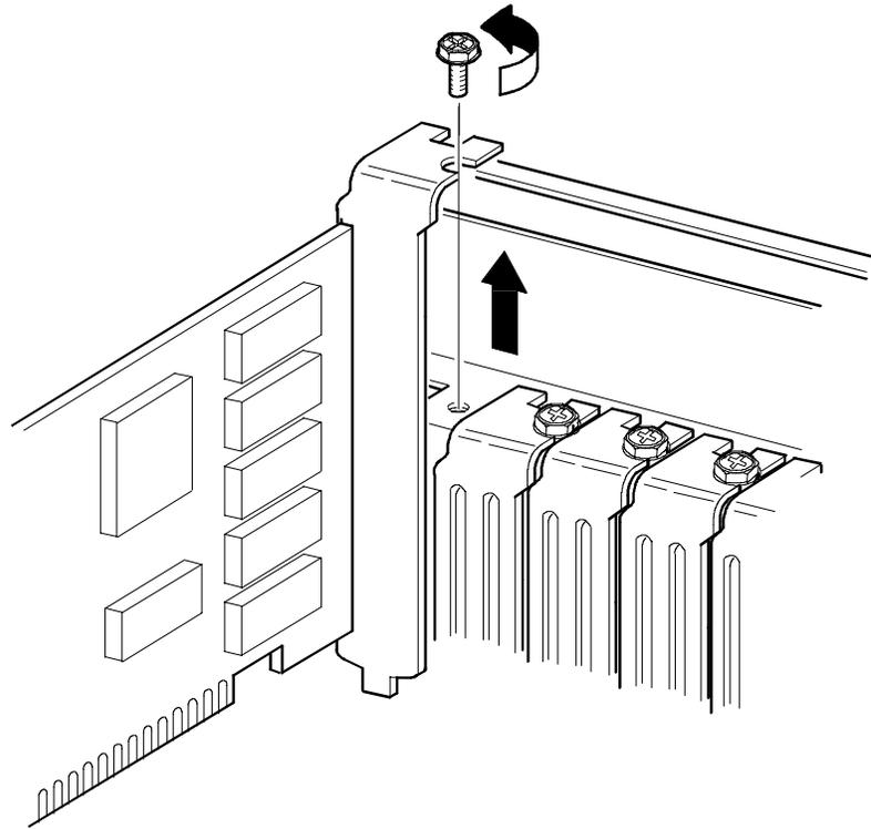
Figure 3 - 9 Removing Expansion Boards
