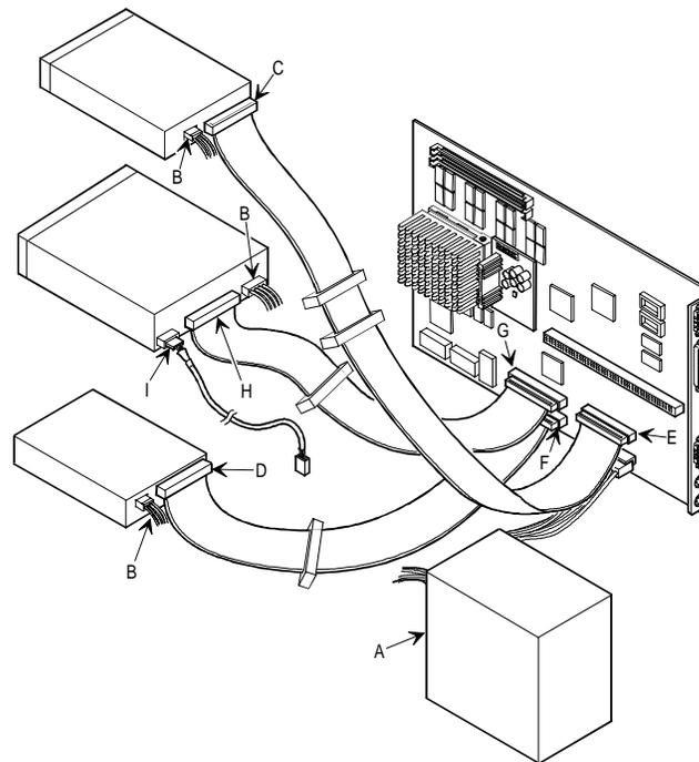
Figure 3 - 14 Diskette and IDE Data Cable Connections
