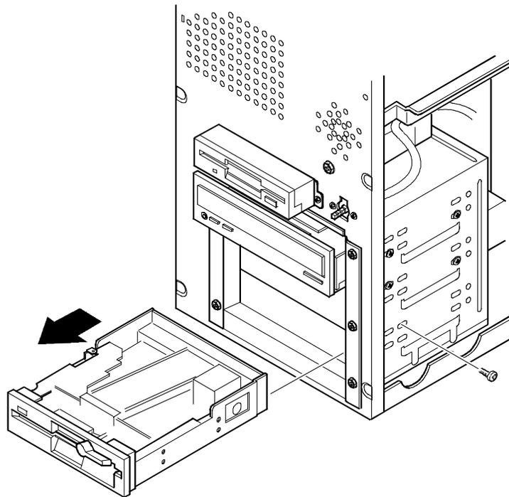
Figure 3 - 7 Removing a 5¼-Inch Device
