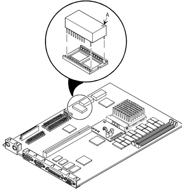
**Figure 3 - 15 Replacing the Computer Battery**
