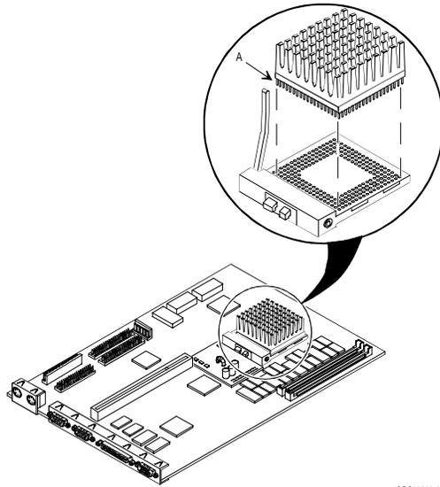
Figure 3 - 13 Installing a Higher Performance CPU
