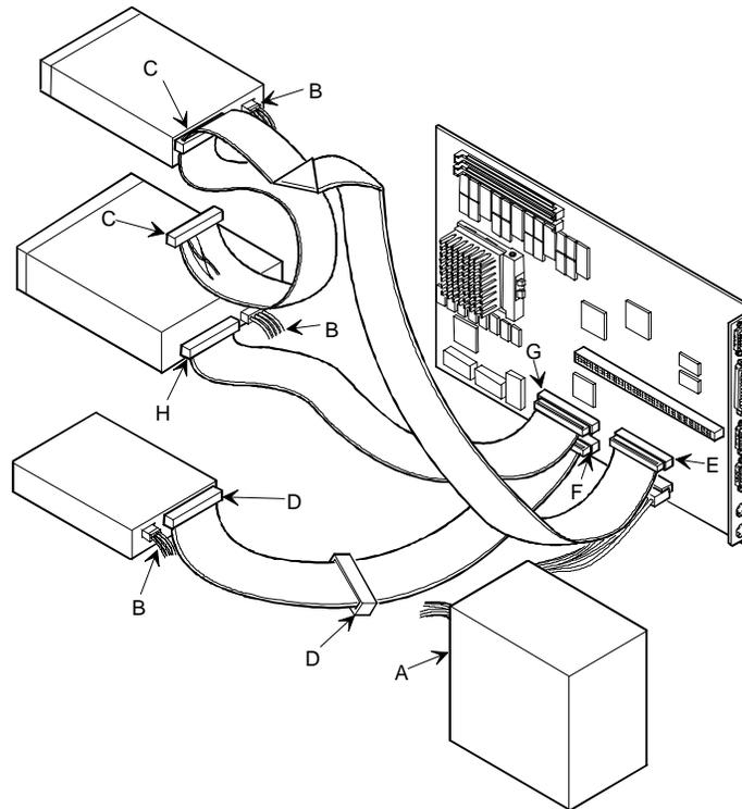
**Figure 3 - 16 Diskette and IDE Data Cable Connections**
