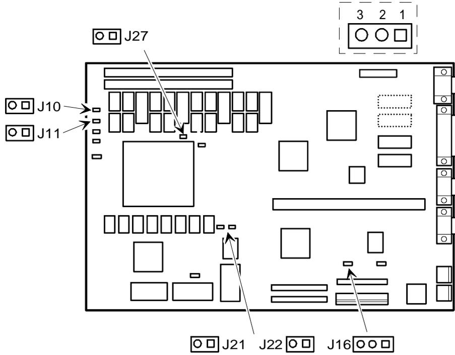
Figure 3 - 4 Main Logic Board Jumper Locations
