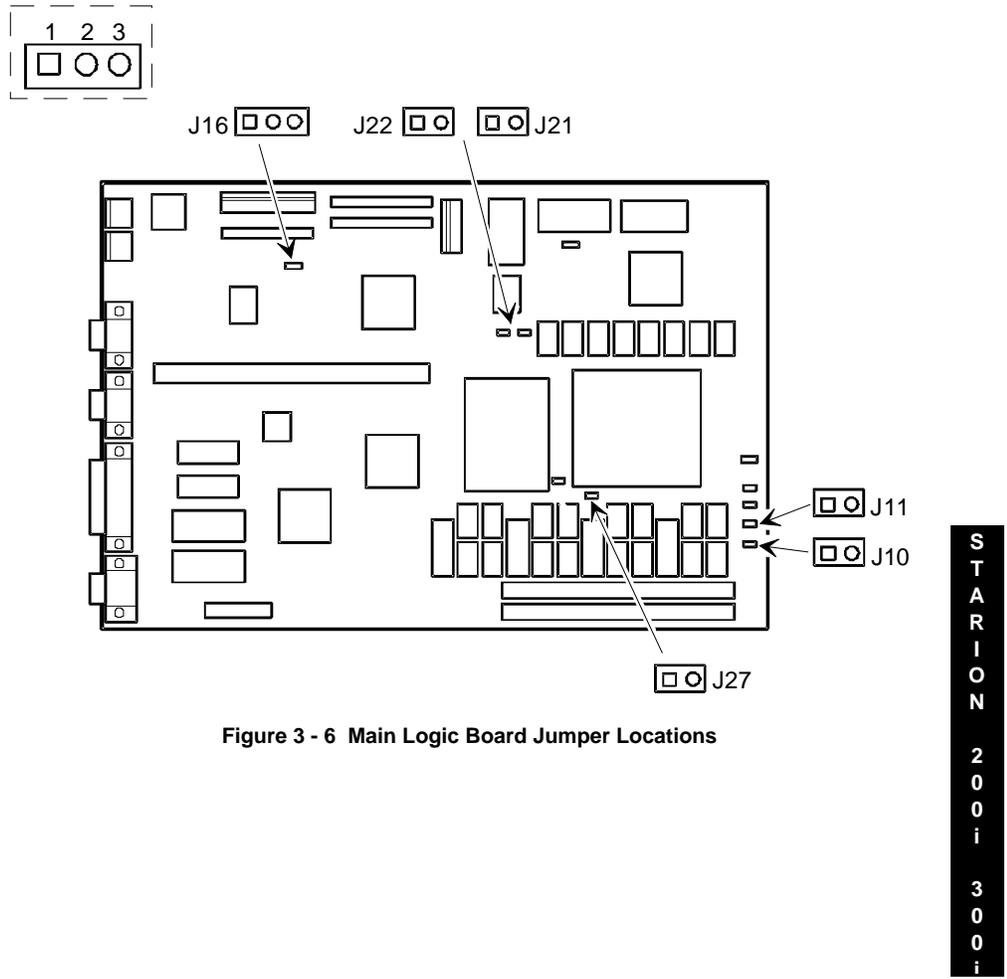
Figure 3 - 6 Main Logic Board Jumper Locations
