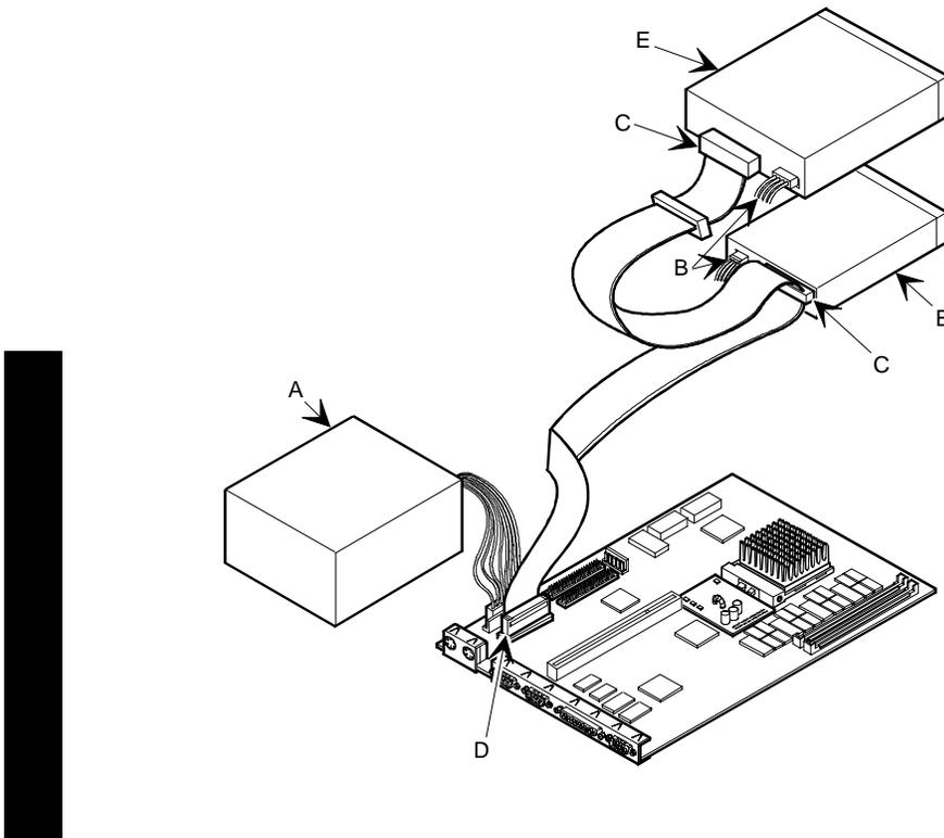
Figure 3 - 19 Diskette Drive Data Cable Connections
