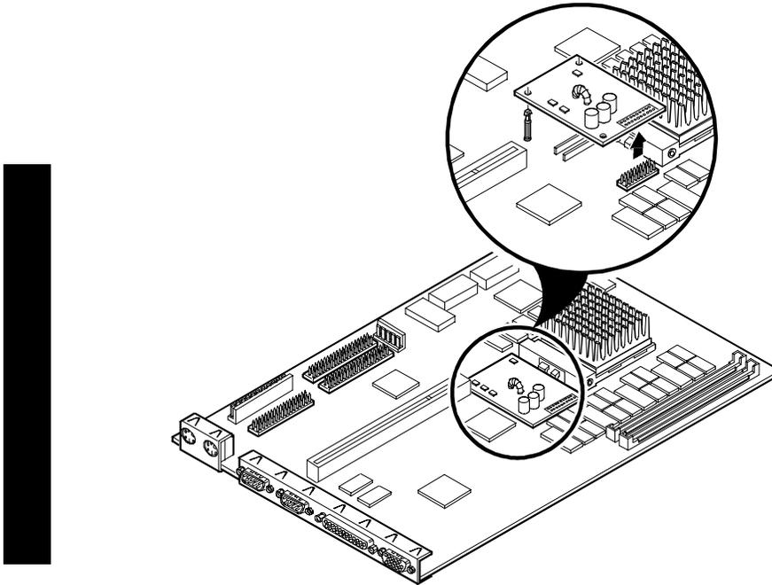
Figure 3 - 17 Installing the CPU Voltage Regulator
