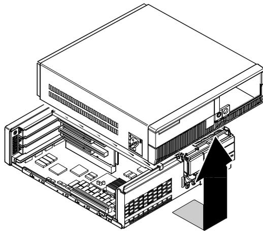
Figure 3 - 3 Removing the Cover
