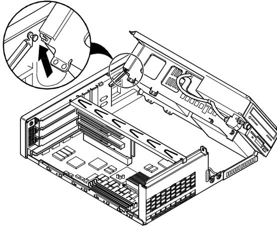
Figure 3 - 14 Open power supply subassembly
