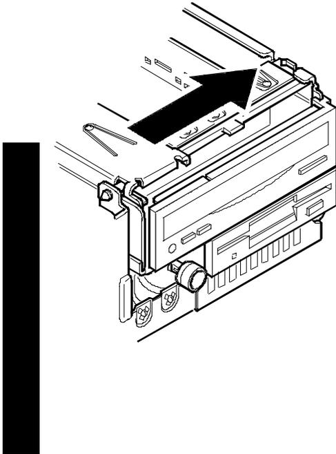
Figure 3 - 8 Release Front Locking Mechanisme
