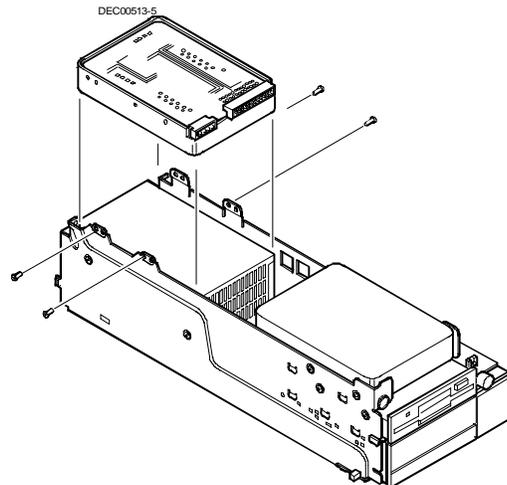
Figure 3 - 15 Removing the 3.5-Inch Device
