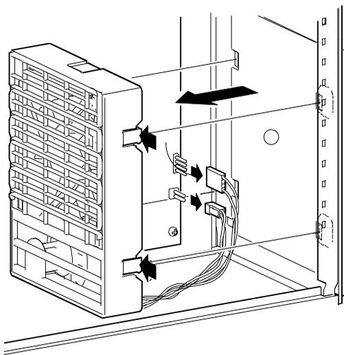
**Figure 3 - 12 Removing the Fan / Speaker Assembly (Pentium)**
