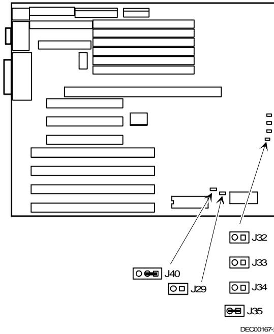
Figure 3 - 5 Main Logic Board Jumper Locations
