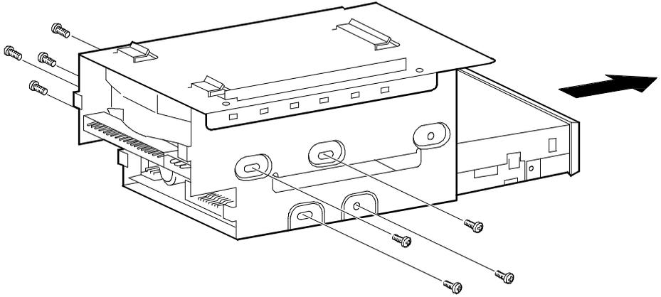
**Figure 3 - 10 Removing the Lower Drive Bay Devices**
