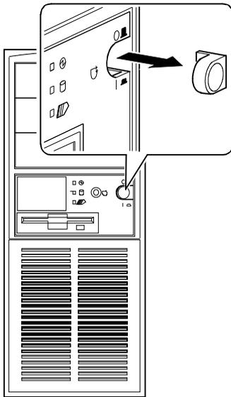
**Figure 3 - 14** Removing the ON/OFF Switch
