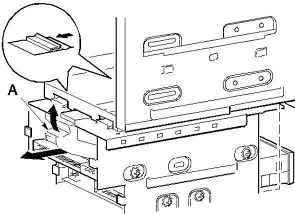
Figure 3 - 9 Removing the Lower Drive Bay Assembly
