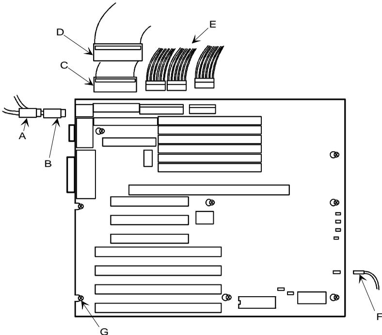
Figure 3 - 11 Removing the Main Logic Board
