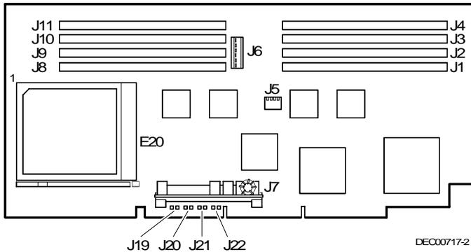
**Figure 3 - 23 CPU Module Component Locations**
