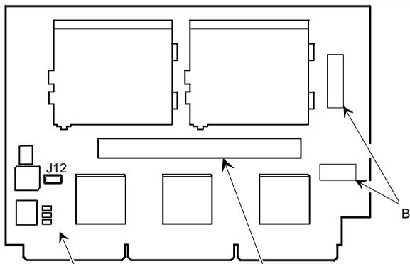
**Figure 3 - 20 Secondary Cache Upgrade Socket and Jumper Locations**
