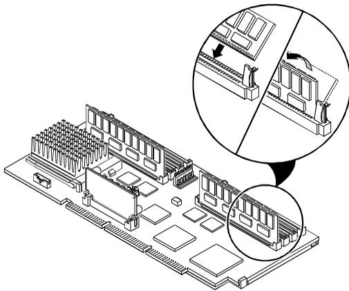
**Figure 3 - 6 Installing a SIMM**
