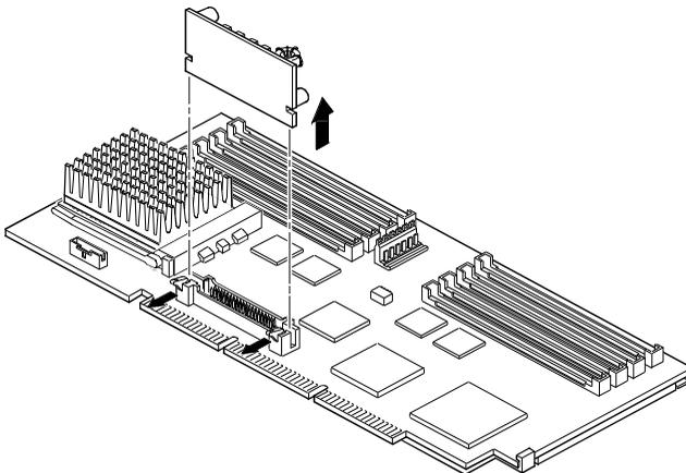
Figure 3 - 25 Voltage Regulator Card
