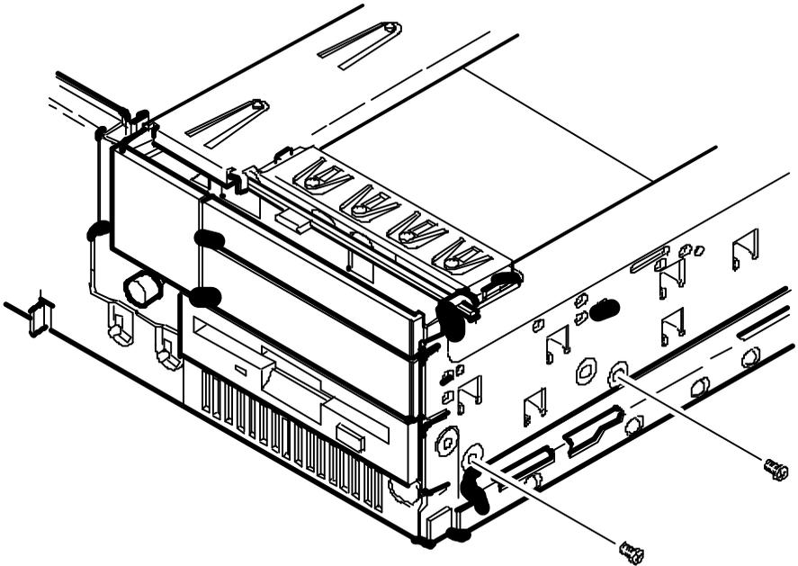
**Figure 3 - 13 Removing the 3½-inch diskette drive (Low-Profile Models)**
