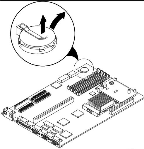
**Figure 3 - 24 Replacing the computer's Battery**
