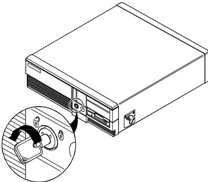
Figure 3 - 1 Unlocking the Cover
