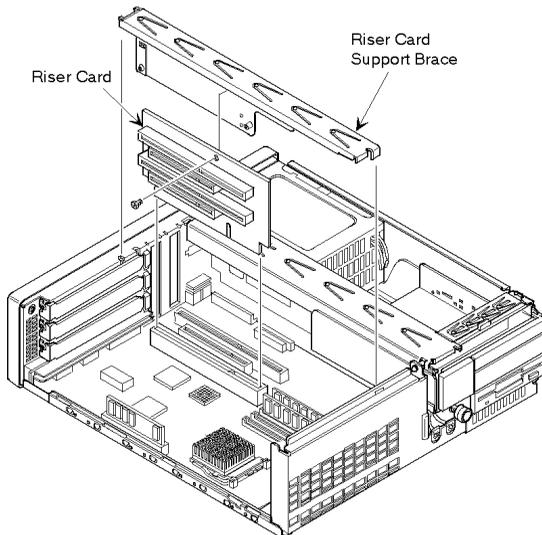
**Figure 3 - 19 Removing the Riser Card & Bracket (Low-Profile Models)**
