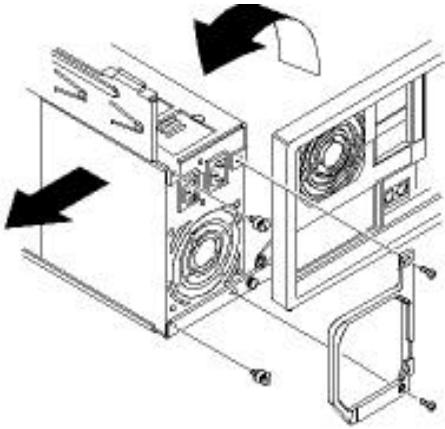
**Figure 3 - 18 Removing the Full-Profile Models Power Supply**
