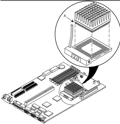
**Figure 3 - 21 Installing a Higher Performance CPU**
