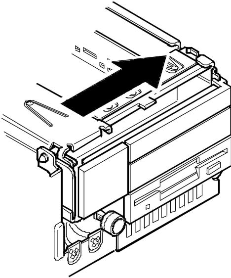
**Figure 3 - 10 Release Front Locking Mechanism**
