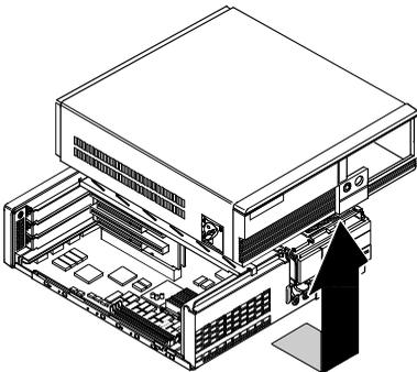
Figure 3 - 3 Removing the Cover
