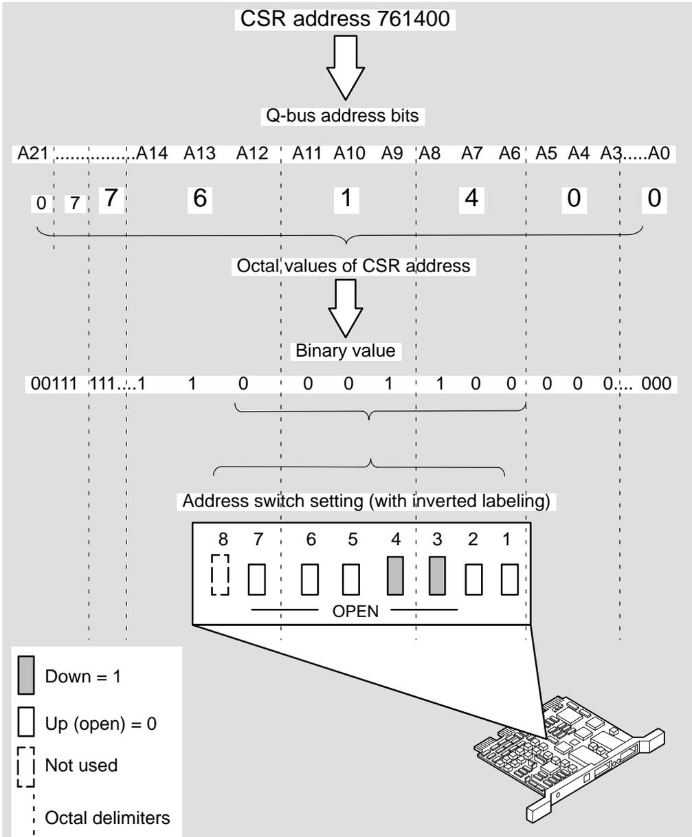
NOTE: The labeling on the switches is shown inverted but is in the proper sequence.
