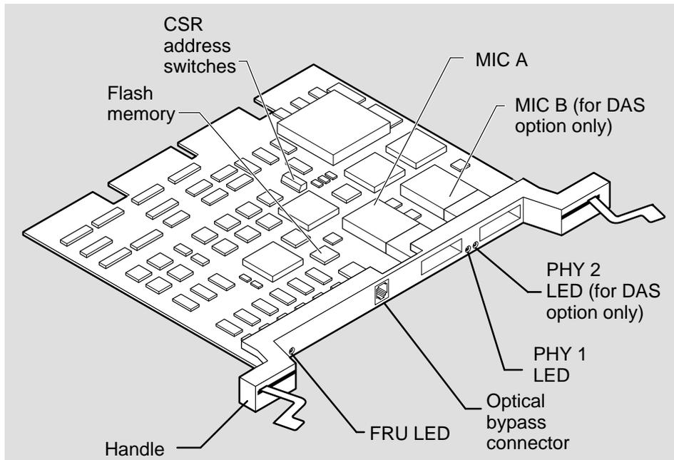
**Figure 1-3: Controller Connectors and LEDs**
