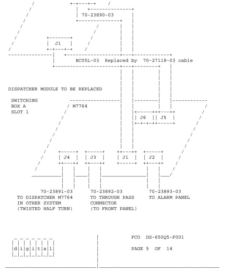
FIELD INSTALLATION AND TEST PROCEDURE FOR FCO DS-650Q5-F001
