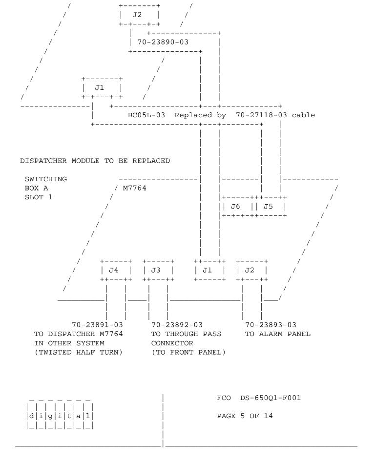
FIELD INSTALLATION AND TEST PROCEDURE FOR FCO DS-650Q1-F001
