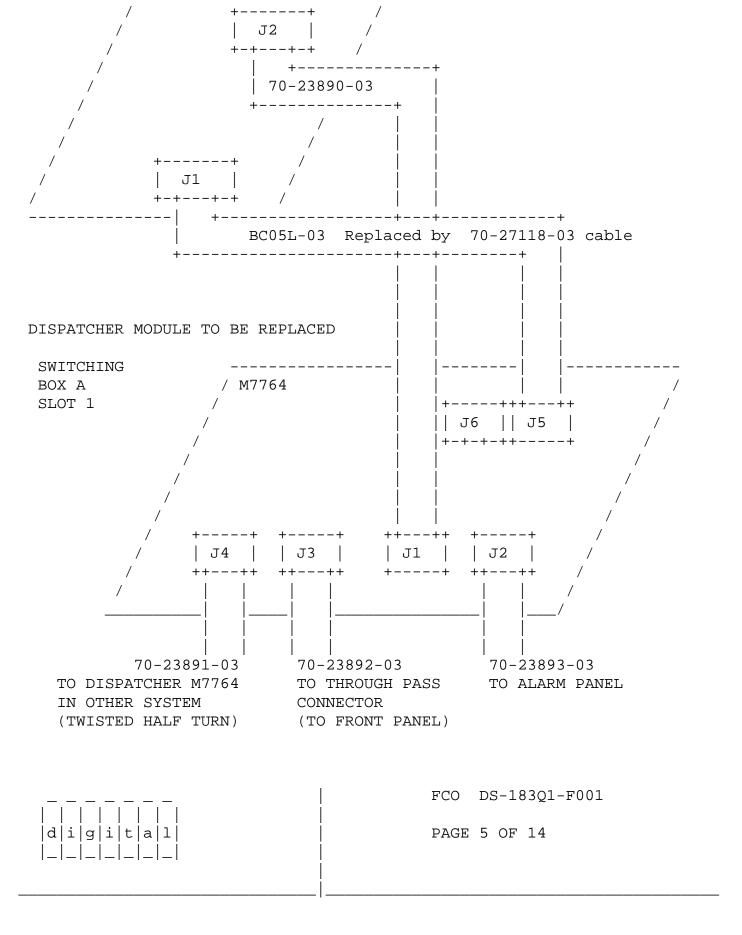
FIELD INSTALLATION AND TEST PROCEDURE FOR FCO DS-183Q1-F001
