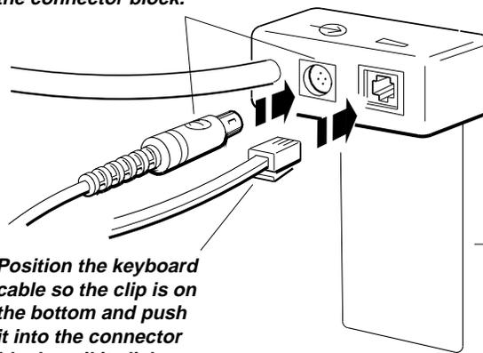
2. *Position the keyboard cable so the clip is on the bottom and push it into the connector block until it clicks into place.*
