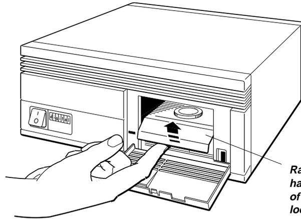
**Raise the insert/release handle behind the bottom of the door until the handle locks into position.**
