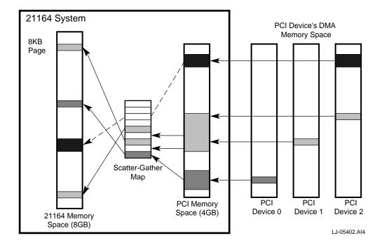
Figure A–17 PCI DMA Addressing Example
