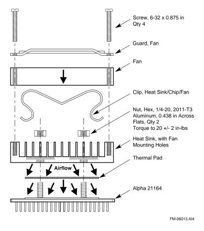
Figure 5–1 Fan/Heat-Sink Assembly
