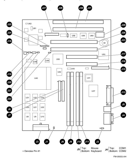
Figure 2–1 AlphaPC 164LX Jumper/Connector/Component Location
