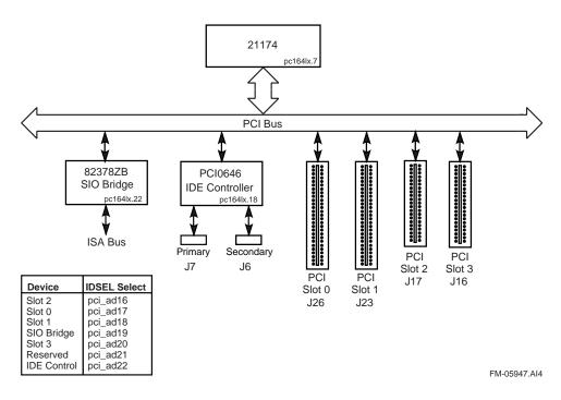
The PCI bus supports multiplexed, burst mode, read and write transfers. It supports synchronous operation of 33 MHz. It also supports either a 32-bit or 64-bit data path with 32-bit device support in the 64-bit configuration. Depending upon
