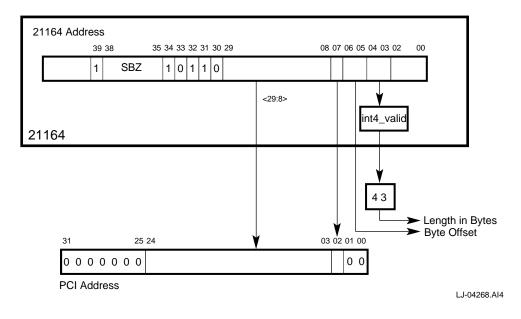
Figure A–12 PCI Sparse I/O Space Address Translation (Region A, Lower 32MB)
