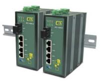
The IFC-1400-X is industrial grade Fast Ethernet Switch that provides 4-port 10/100Base-TX and 1-port 100Base-FX. The reliable hardware design is suitable for keeping industrial automation application running continuously. Each IFC-1400-X media converter comes with two relay output alarms and two redundant DC power inputs to help prevent damage and loss. The IFC-1400-X media converter is available in models that support operating temperatures of -40 to 85 degree C.
