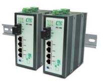
The IFC-1400 is industrial grade Fast Ethernet Switch that provides 4-port 10/100Base-TX and 1-port 100Base-FX. The reliable hardware design is suitable for keeping industrial automation application running continuously. Each IFC-1400 media converter comes with two relay output alarms and two redundant DC power inputs to help prevent damage and loss. The IFC-1400 media converter is available in models that support operating temperatures of 0 to 60 degree C.
