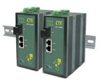
The IFC-1200-X is industrial grade fiber media converter that provides 2-port 10/100Base-TX and 1-port 100Base-FX. The reliable hardware design is suitable for keeping industrial automation application running continuously. Each IFC-1200-X media converter comes with two relay output alarms and two redundant DC power inputs to help prevent damage and loss. The IFC-1200-X media converter supports operating temperatures of -40 to 85 degree C.
