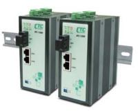
The IFC-1200 is industrial grade fiber media converter that provides 2-port 10/100Base-TX and 1-port 100Base-FX. The reliable hardware design is suitable for keeping industrial automation application running continuously. Each IFC-1200 media converter comes with two relay output alarms and two redundant DC power inputs to help prevent damage and loss. The IFC-1200 media converter supports operating temperatures of 0 to 60 degree C.
