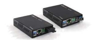
The FMC-1000E is a copper to fiber Gigabit Ethernet solution designed to make conversion between 10/100/1000Base-TX and 1000Base-SX/LX. The FMC-1000ES provides the fiber gigabit with SFP connector. This non-managed converter has a simple DIP switch for setting auto or forced mode and for enabling or disabling its LFP (Link Fault Pass-thru) feature.
