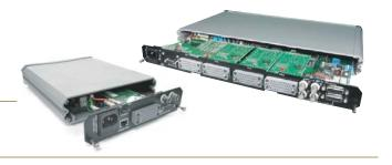
When purchasing one of our single or multi-port access units or multiplexers that support user replaceable interface modules, our ETU/TTU interface modules provide easily selectable electrical interfaces for a wide selection of user applications. In addition to standard datacom interfaces such as V.35, RS-530, X.21, RS-449, etc. Ethernet modules are also available for bridging or routing of Ethernet over E1 or T1 network services.
