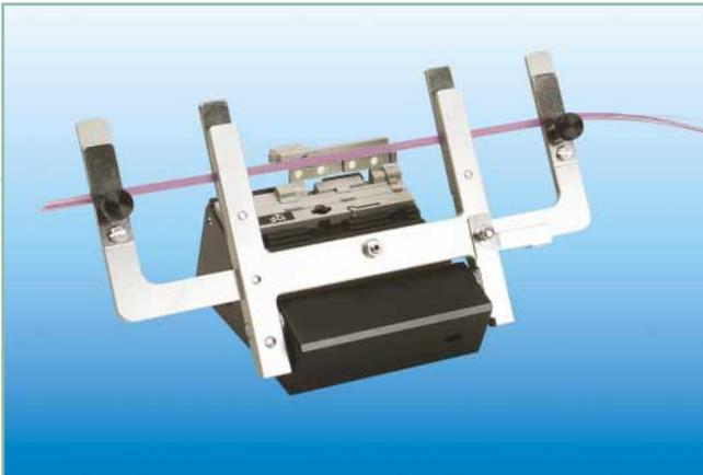
*Ribbonizer with inserted handling adapter for 1 to 12 fibers*
