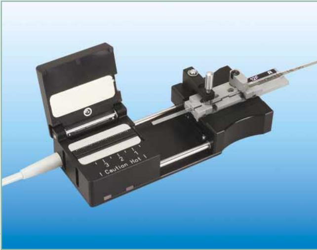
*Thermal Stripper with inserted handling adapter*
