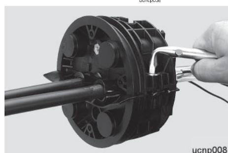
**5.4** Fit upper half of end cap, press it down and using the accompanying screws and washers **slowly** close it by tightening the screws alternately until the closing gage fits.
