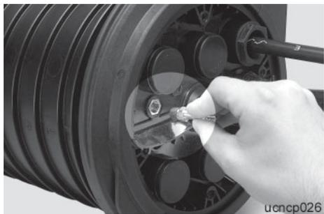
**11.8** Insert valve, grounding screw or closing screw if necessary. Before inserting, lubricate the thread of the valve or screw with sealing paste and let dry.
