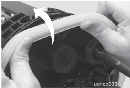
**11.4** Place the sealing ring on the outer edge of the end cap and press it in the sealing slot ...
