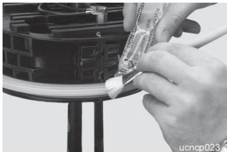
**11.5** For easy closing, the closure can be positioned vertically. Apply lubricant to both sides of the sealing ring.
