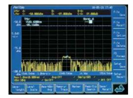
The SNR is improved by using averaging processing. The following is an example of measurement result after 10 sweep averaging are performed.
