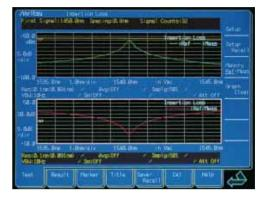
In addition, the measurement results for a specified WDM channel wavelength can be displayed as a list.
