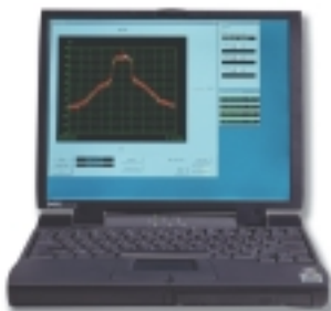
An example of the ACPR measurement result as seen on the PA Navigator.
