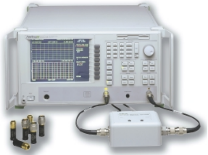
Easy 2-port calibrations using AutoCal ® .
