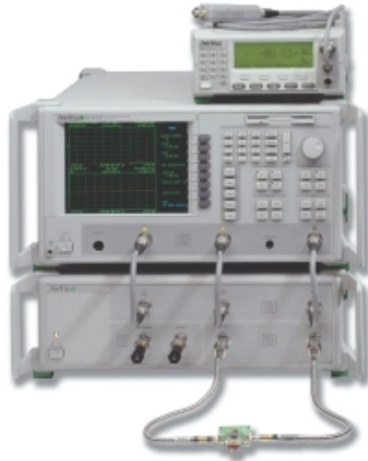
The complete test setup for power amplifier measurements with a single connection.
