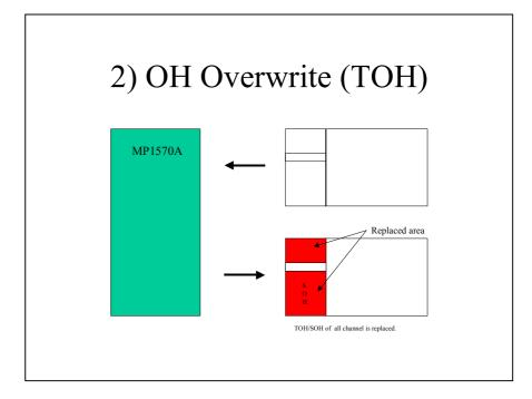
In the POH overwrite mode, the POH is changed to an internally generated pattern. The delay at POH overwrite is detected and the STS/Au pointer is replaced automatically.
