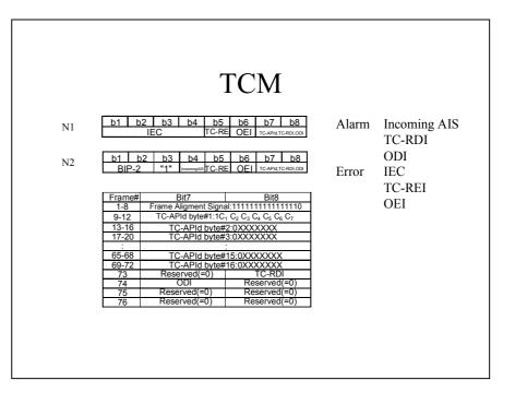
In addition to measuring TC errors and alarms dynamically, the MP1570A SONET/SDH/PDH/ATM Analyzer can also set and monitor the TC-APId.
