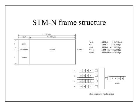
SOH is the overhead for monitoring the section. The MP1570A SONET/SDH/PDH/ATM Analyzer can access all SOH bytes. It can also generate and measure pseudoalarms and -errors in the section. In addition, it can perform BER measurement of overhead bytes.
