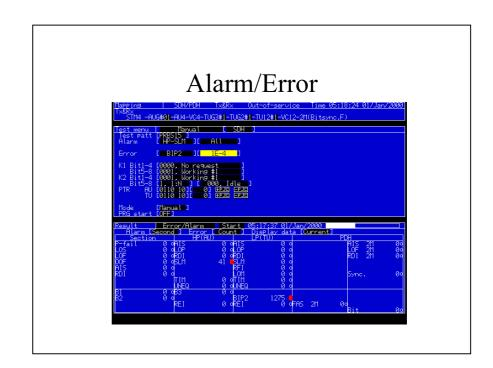
The ITU-T recommendations specify various error performance standards; parameters used by SDH are specified by G.826. The MP1570A SONET/SDH/PDH/ATM Analyzer supports all these error performance standards, and can also perform measurement according to the earlier G.821 specifications.
