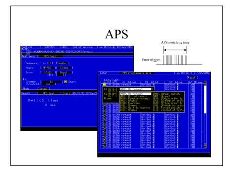
The SONET/SDH equipment communicates alternately using K1/K2 and performs switching, etc., automatically. The MP1570A SONET/SDH/PDH/ATM Analyzer can generate the K1/K2 sequence and can capture the received sequence.
