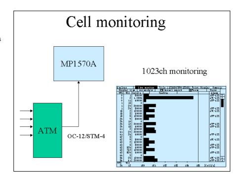
At 1-point CDV delay time measurement, the CBR cell delay (variation) is measured. The measured actual arrival time is compared to the estimated arrival time. The results indicating the cell delay trend are displayed as a graph.
