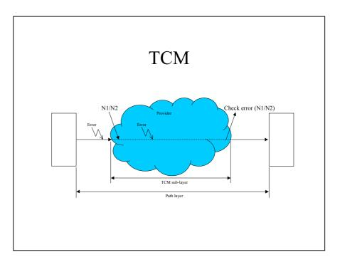
The N1/N2 bytes are not used just for error monitoring; they also include various functions for sending alarms, etc.
