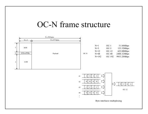
In SONET, the basic OC-1 (52 Mbps) rate is multiplexed and the MP1570A SONET/SDH/PDH/ATM Analyzer can measure up to OC-192.
