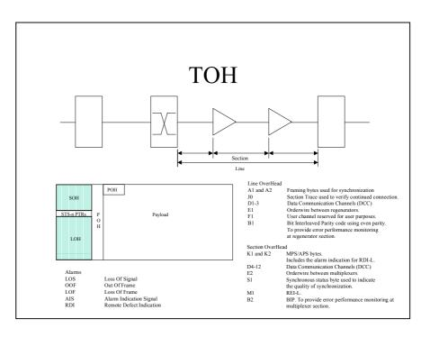
STS POH is the overhead for monitoring the STS path section. The MP1570A SONET/SDH/PDH/ ATM Analyzer can access all STS POH bytes. It can also generate and measure pseudo-alarms and -errors in the STS path section. In addition, it can perform BER measurement of overhead bytes.
