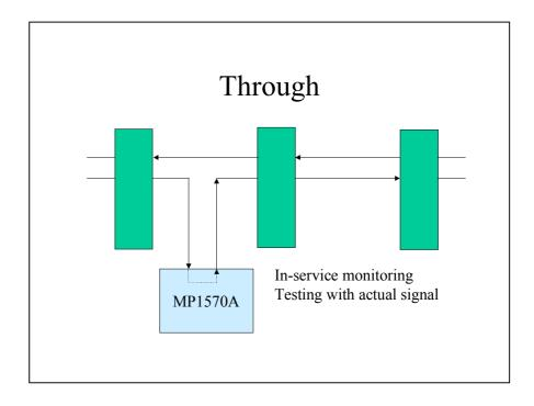
The MP1570A SONET/SDH/PDH/ ATM Analyzer can select various Through configurations, such as Transparent Through, OH Overwrite, and Payload Overwrite; it can access a specific channel and can insert an internally generated test signal.
