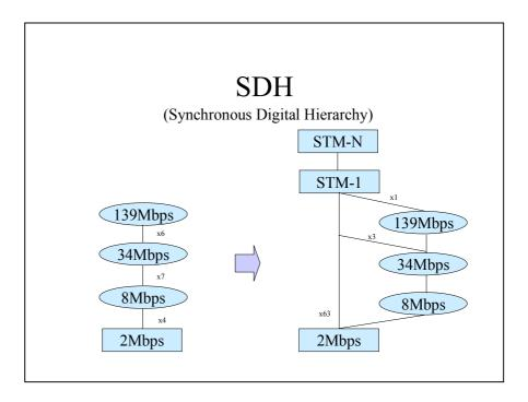
In SDH, the basic STM-1 (156 Mbps) rate is multiplexed and the MP1570A SONET/SDH/PDH/ATM Analyzer can measure up to STM-64.
