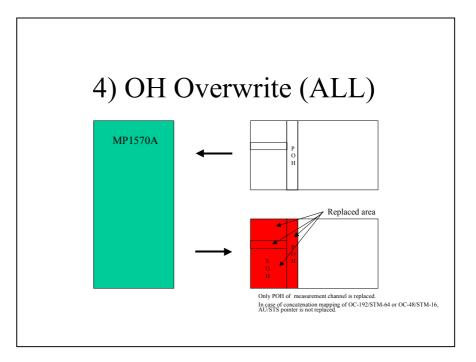
The payload can also be overwritten. A test signal can be inserted into the selected channel and BER measurement can be performed. The pointer is adjusted automatically according to the delay, thereby eliminating concerns about delayrelated errors.
