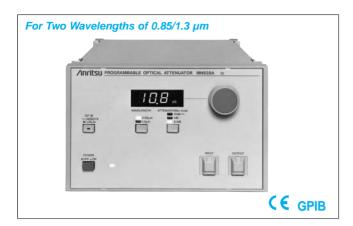
The MN938A can set attenuation in a range of 0 to 60 dB in 0.1 dB steps. Two wavelengths can be selected. As the MN938A is provided with GPIB as standard, it can be used in a variety of automatic measuring systems for development, production, and inspection. A rotary encoder permits attenuation to be set smoothly even when used manually.
