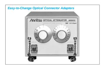
The MN9605C is high-precision optical attenuators designed for use with single mode optical fibers. A combined step attenuator and continuous attenuator permit highly accurate attenuation adjustment. The MN9605C has PC-type optical connectors, so that internally-reflected light is thoroughly suppressed. It is precisely constructed for single-mode fiber use and can be used as a highly accurate 65 dB variable attenuator.
