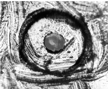
Figure 5-10. Damage from improper cleaning.
