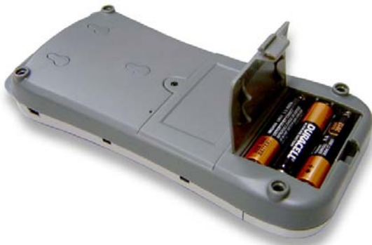
ACR88U back side showing the 3 AAA battery slots
